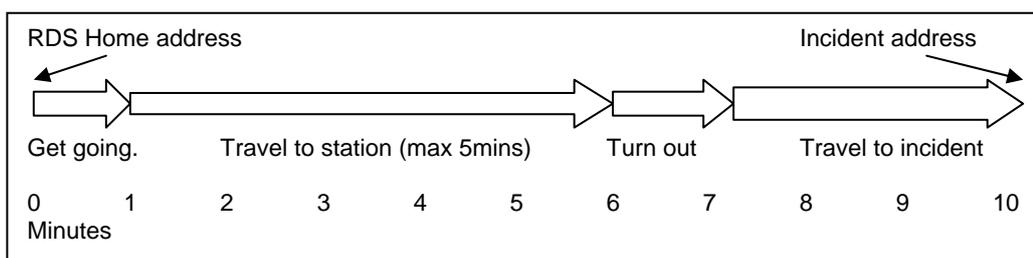
Figure 4 – pictorial representation of (10 minute) travel times to incident
