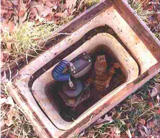
Photograph showing typical data logger installation with hydrant cap and flexible hose
