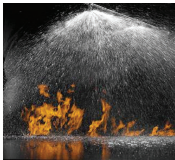
An example of a domestic sprinkler activating to demonstrate the amount of spray produced
