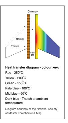
Over a period of time the temperature of the thatch chimney interface can become critical (approx. 200°C) and lead to a chain of events that cause a thatch fire.
